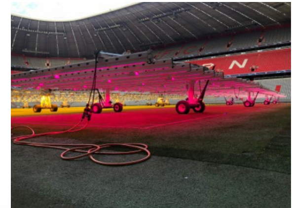
Figure 48: Led lights for optimal grass growth at Allianz Arena (Munich). Source: https://www.stadia-magazine.com/news/field-lighting/allianz-arena-first-to-use-led-lights-to-grow-turf.html#prettyPhoto
