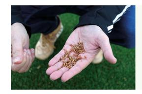
The birch-pitch (Pitch A) is one of four new training pitches at Sukkevann Stadium. Pitch B has pure sand infill. The last two (C & D) have crumb rubber infill, the most common infill in Norway. This way we will see the comparisons between the different materials during the season.
